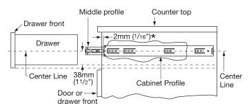
• Attach drawer profile portion of the slide to the side of the drawer on centerline as illustrated with the appropriate screws.
