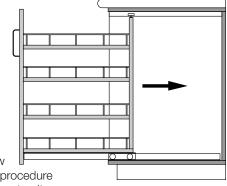
Pull-out unit is now installed. Reverse procedure to remove the Pull-out unit.
