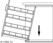
**3.** Allow Pull-out unit roller to drop down behind bottom cabinet roller and lean unit forward.
