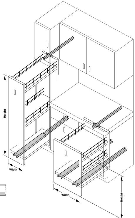
On taller units it may be necessary to thru-bolt the pull-out to the slide as illustrated below. Use 1/4-20 flathead bolts and nuts.
