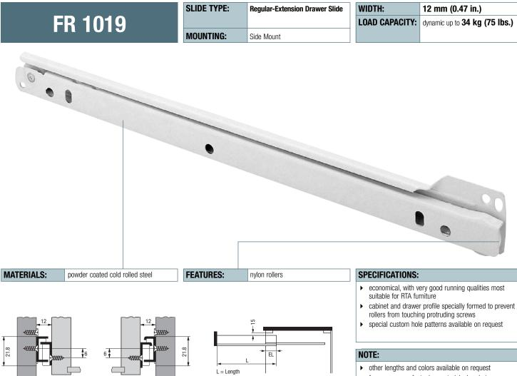
12 mm (0.47 in.) is the actual size of the slide. Allow a min. of 12.7 mm (0.5 in.) for clearance. EL = Extension Loss
